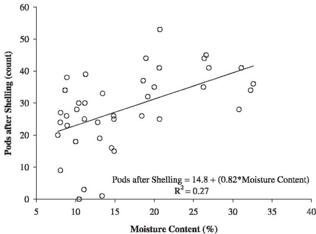
Fig. 1. Comparison of moisture content and unshelled pod count for shelling with the grade sheller with pod recycling.
