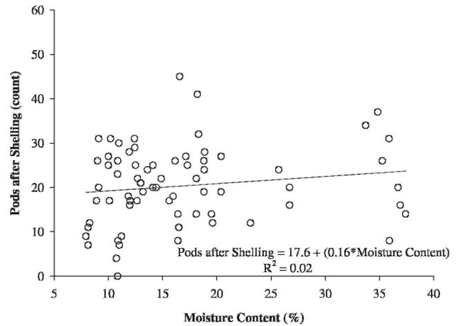
Fig. 2. Comparison moisture content and unshelled pod count for shelling with the grade sheller without pod recycling.
