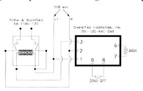
Fig. 1. Schematic of a screen vibrator timing device with a mechanical relay.
