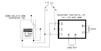
Fig. 2. Schematic of a screen vibrator timing device with a solid state relay.
