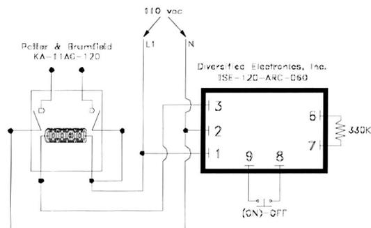
Fig. 1. Schematic of a screen vibrator timing device with a mechanical relay.
