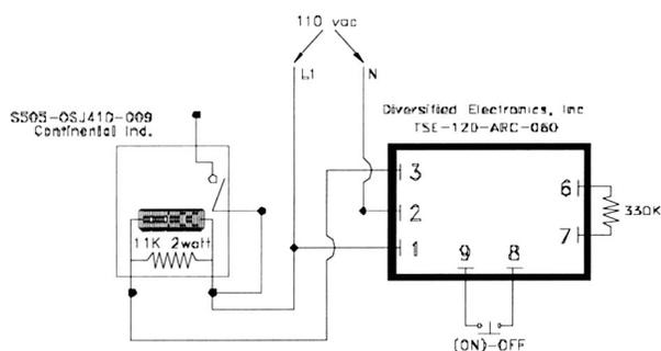
**Fig. 2. Schematic of a screen vibrator timing device with a solid state relay.**
