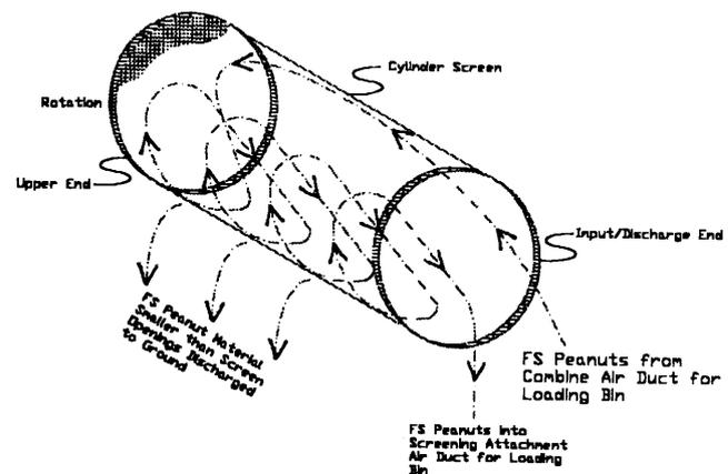
Fig. 2. A schematic of farmer stock peanut material movement during trommel operation.
