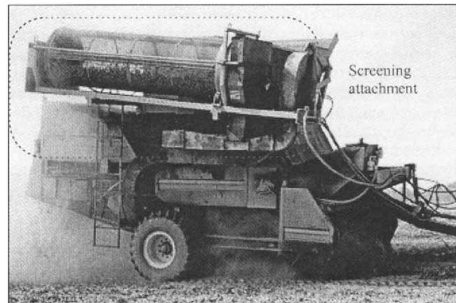
Fig. 1. The screening attachment installed on an Amadas peanut combine.
