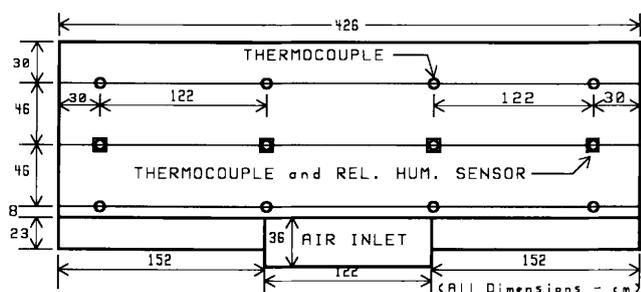
Fig. 1. Side view showing position of temperature and relative humidity sensors in the wagons and boxes.
