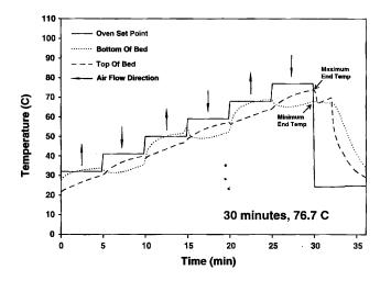
Fig. 2. Peanut bed temperatures during the 30 min/76.7 C maximum temperature blanching protocol.
