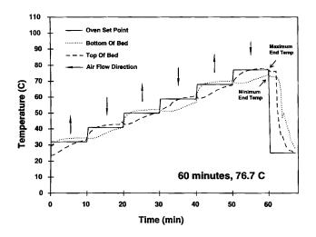
Fig. 3. Peanut bed temperatures during the 60 min/76.7 C maximum temperature blanching protocol.
