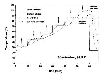
Fig. 5. Peanut bed temperatures during the 60 min/98.9 C maximum temperature blanching protocol.
