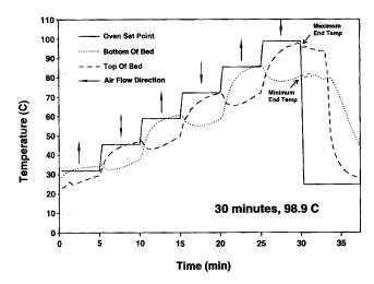
Fig. 4. Peanut bed temperatures during the 30 min/98.9 C maximum temperature blanching protocol.
