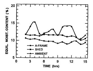
Fig. 4. Equilibrium moisture content for ambient and headspace of covered containers for the 1993 storage period.
