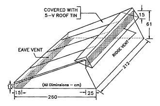
Fig. 1. Shed cover for half-trailer container.
