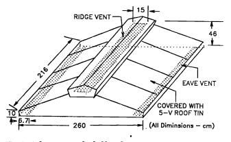
Fig. 2. A-frame cover for half-trailer container.
