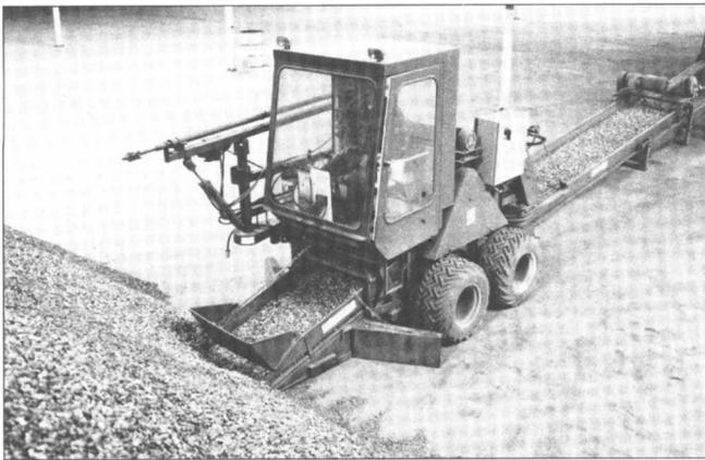
Fig. 1. Spudnik Potato Scooper with accompanying potato conveyors.
