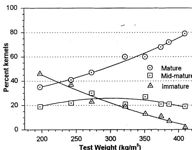
Fig. 7. Effect of in-shell test weight on maturity distribution of shelled-stock kernels. Water-stressed "medium" runners.
