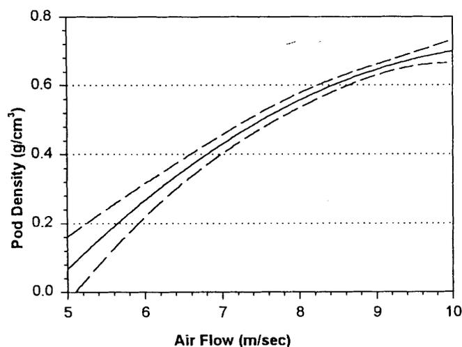
Fig. 3. Regression analysis between pod density ( $\text{g/cm}^3$ ) and air flow ( $\text{m/sec}$ ) required to float Florunner peanut pods. 95% confidence interval shown.  $R^2=.58$ .
