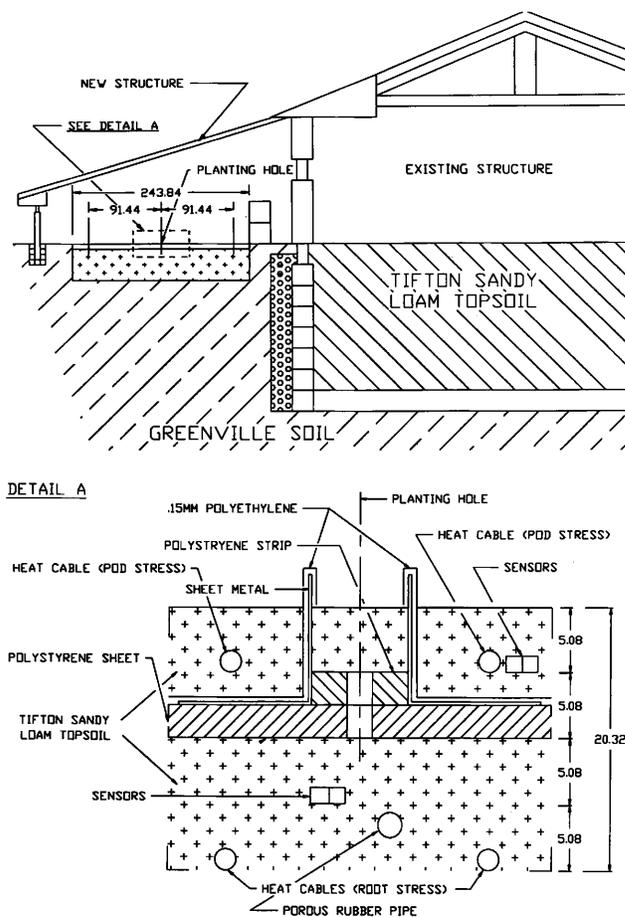
Fig. 1. Cross sectional view of plots used to separate peanut pod zone and root zone drought stress. Dimensions are cm unless otherwise indicated.
