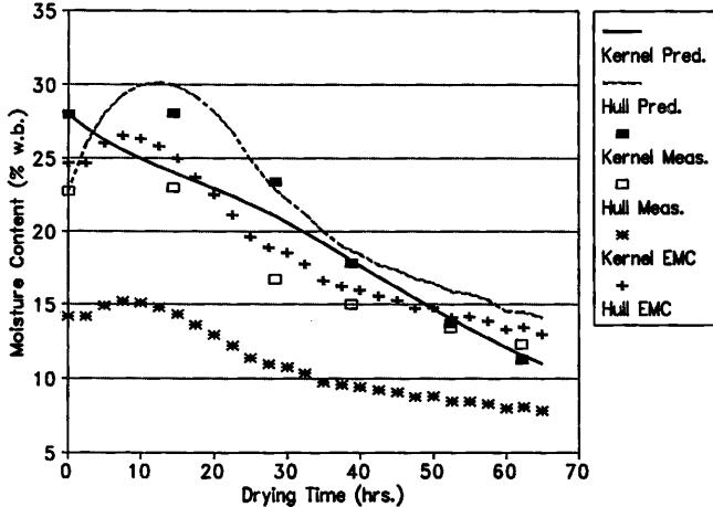
Fig. 2. Drying curves for the top layer of wagon number 11 from 1989 drying experiments.
