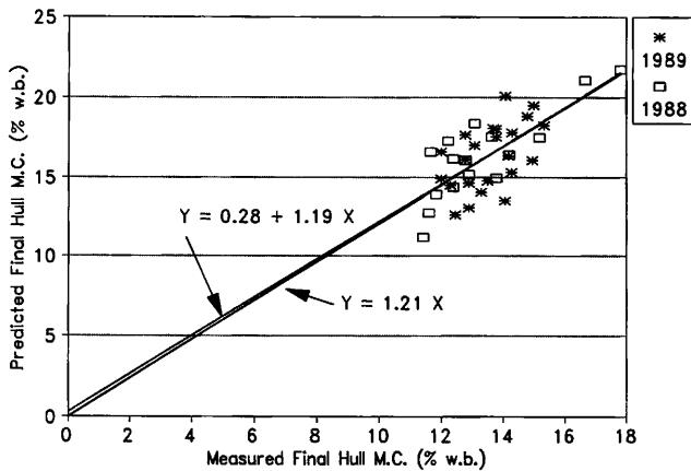
Fig. 11. Comparison of predicted and measured final hull moisture contents at top of peanut wagons during 1988 and 1989.
