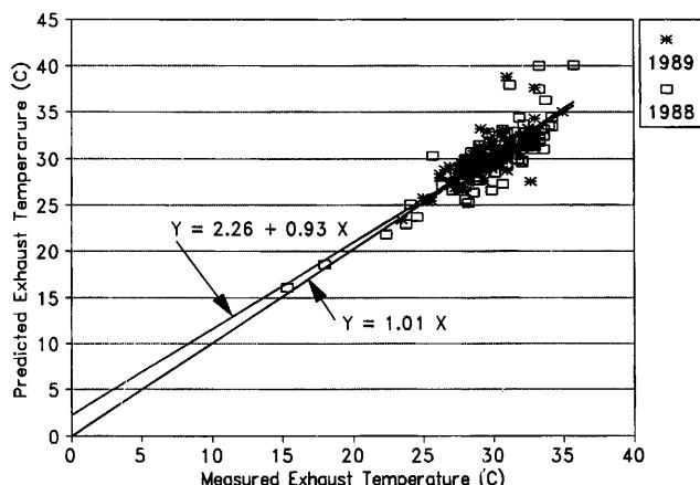
Fig. 8. Comparison of predicted and measured exhaust air temperatures for wagon drying studies of 1988 and 1989.
