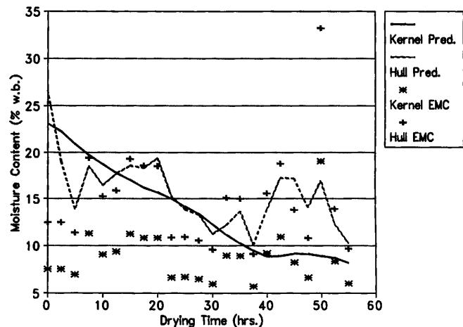
Fig. 5. Drying curves for the bottom layer of wagon number 46 of the 1989 drying experiments.
