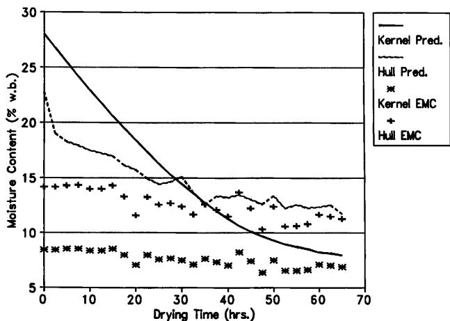
Fig. 1. Drying curves for the bottom layer of wagon number 11 in 1989 experiments.
