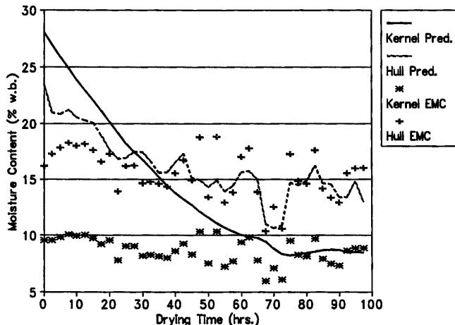
Fig. 3. Drying curves for the bottom layer of wagon number 21 of the 1989 drying experiments.
