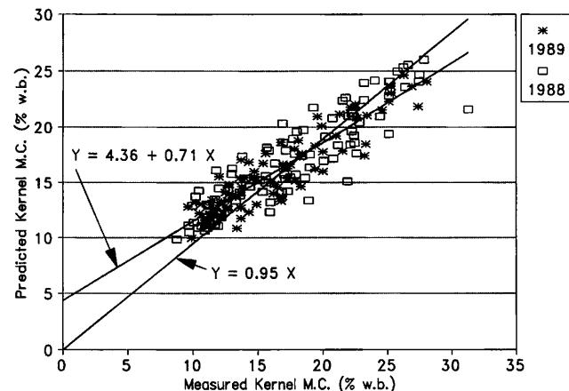
Fig. 9. Comparison of predicted and measured kernel moisture contents at the top of drying wagons during 1988 and 1989.
