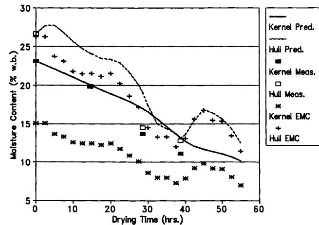
Fig. 6. Drying curves for the top layer of wagon number 46 of 1989 drying experiments.
