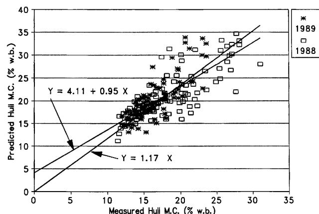
Fig. 10. Comparison of predicted and measured hull moisture contents at top of peanut drying wagons in 1988 and 1989.
