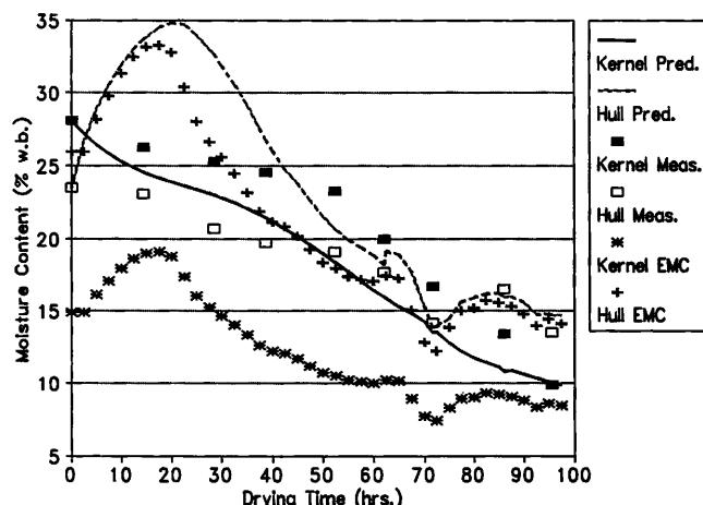
Fig. 4. Drying curves for the top layer of wagon number 21 of the 1989 drying experiments.
