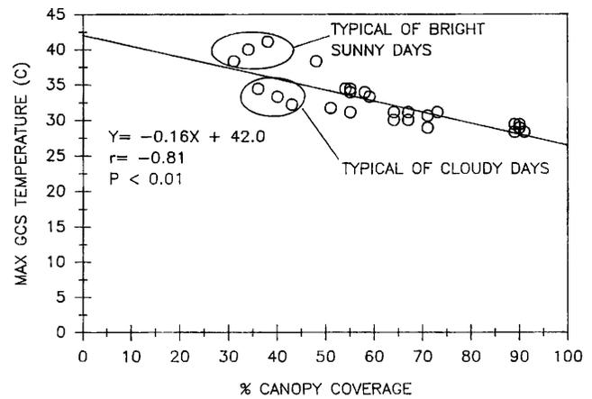
**Fig. 1. Typical relationship of maximum GCS temperature to canopy coverage in absence of plant stress.**
