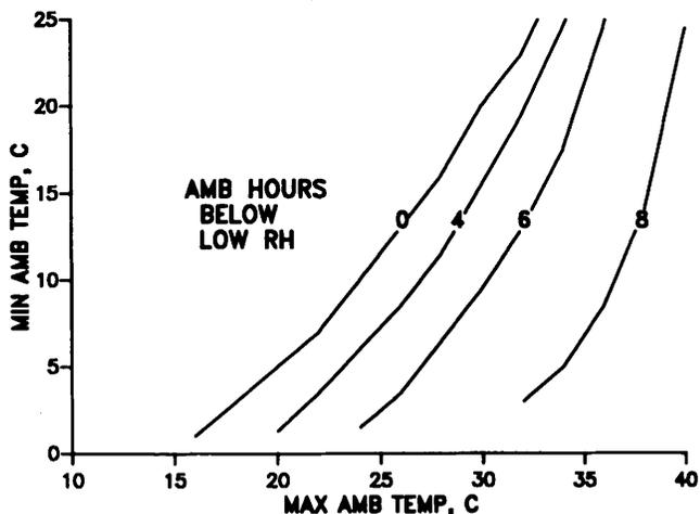
Fig. 4. Time that ambient RH is less than the recommended limit.
