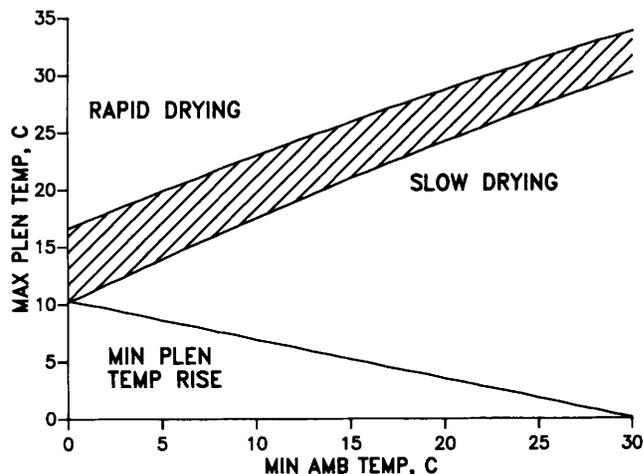
Fig. 5. Maximum plenum temperature and plenum temperature rise based on minimum ambient temperature.
