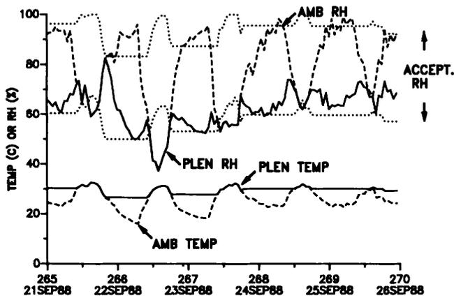
Fig. 7. Plenum temperature control based on actual ambient conditions (high ambient temperatures).
