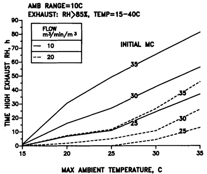
Fig. 8. Time that exhaust RH exceeds 85% with airflow and initial moisture.
