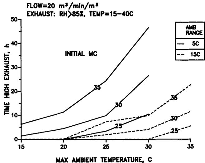
Fig. 9. Time that exhaust RH exceeds 85% with initial moisture and ambient temperature range.
