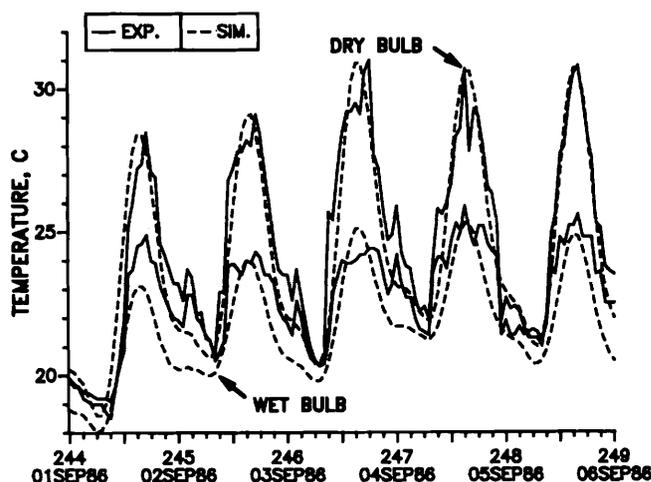
Fig. 1. Experimental and simulated ambient temperatures.
