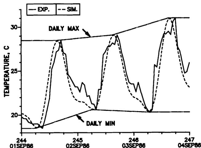
Fig. 2. Max and min temperatures used to calculate simulated hourly ambient dry bulb temperatures.
