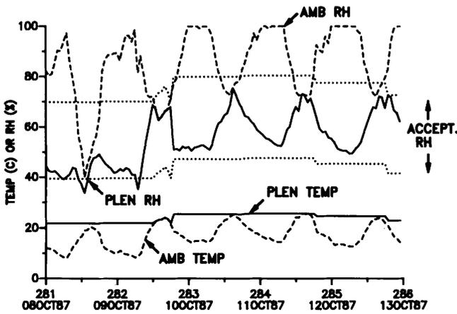
Fig. 6. Plenum temperature control based on actual ambient conditions (low ambient temperatures).
