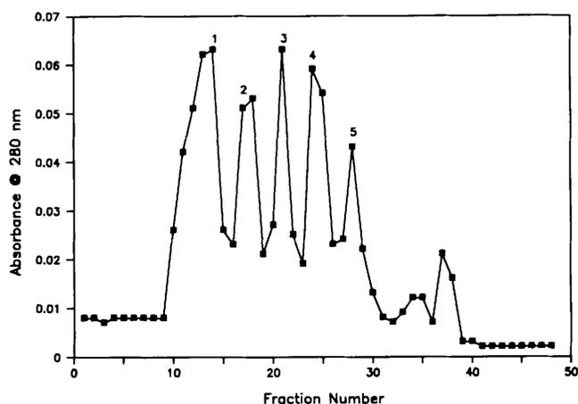
Fig. 1. Size exclusion chromatography. Sephadex G-50 column equilibrated with 6 M guanidine hydrochloride containing 0.01 M mercaptoethanol which was also used as a mobile phase. Peaks 1-5 represent fractions exhibiting antitryptic activity.
