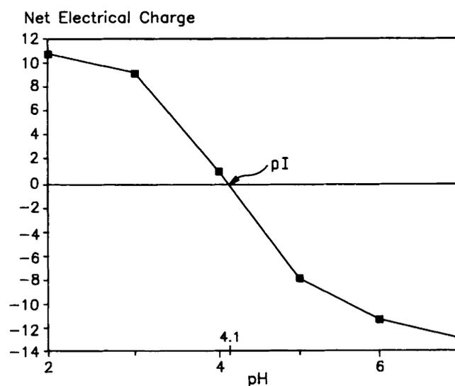
Fig. 4. Net electrical charges for aspartic acid, glutamic acid, lysine, histidine and arginine at different pH's. pI is the pH where the net charge = 0.
