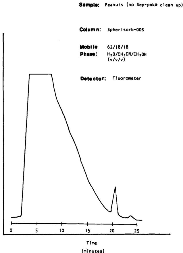
Fig. 5. Chromatogram of peanut extract with no Sep-pak® cleanup.
