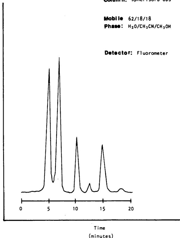
Fig. 2. Chromatogram of aflatoxin standard.
