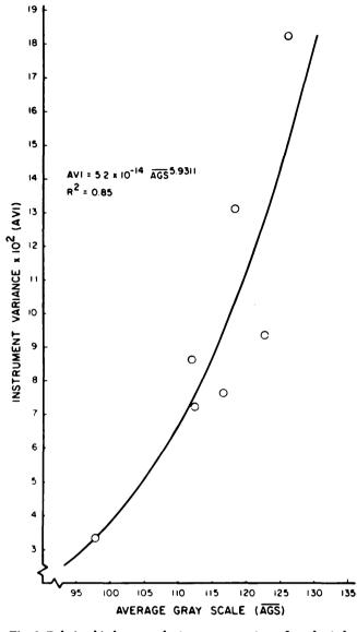
Fig. 6. Relationship between the instrument variance for color index AVI and the average gray scale ACS when making one measurement on a 33.6 cm<sup>2</sup> area of peanut butter. Coefficient of determination  $R^2 = 0.85$ .
