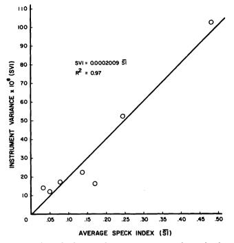
Fig. 4. Relationship between the instrument variance for speck index SVI and the average speck index SI when making one measurement on a 33.6 cm<sup>2</sup> area of peanut butter. Coefficient of determination  $R^2 = 0.97$ .
