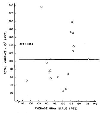
Fig. 5. Relationship between the total variance for color index AVT and the average color index AGS when measuring 33.6 cm<sup>2</sup> area of peanut butter.
