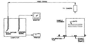
Fig. 1. Schematic diagram of the video image capture system.
