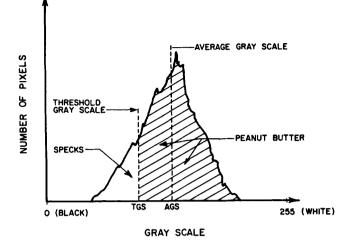
Fig. 2. Typical frequency distribution showing the number of picture elements (pixels) at various shades of gray.
