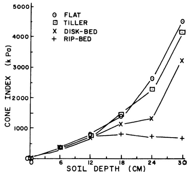
Fig. 1. Average cone index values with soil depth for four seedbed preparations (soil moisture content, 10-12% d.b., Suffolk, VA).
