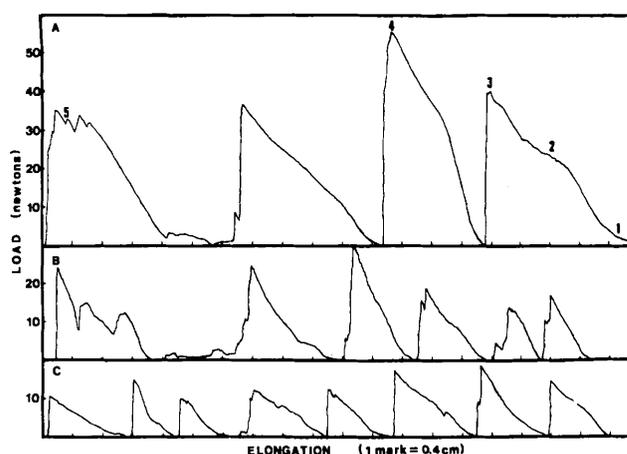
Fig. 1. Peg detachment curves as recorded by the Instron test instrument. A) Curves from pegs of cultivar PI 393647 (strong group); B) Curves from pegs of cultivar PI 306228 (moderate group); C) Curves from pegs of cultivar PI 365553 (weak group).
