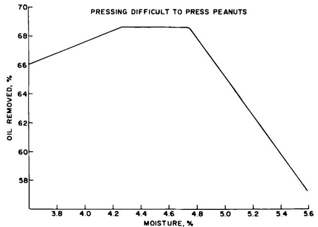
Fig. 2. Effects of moisture on removal of oil from Difficult-to-Press peanuts.
