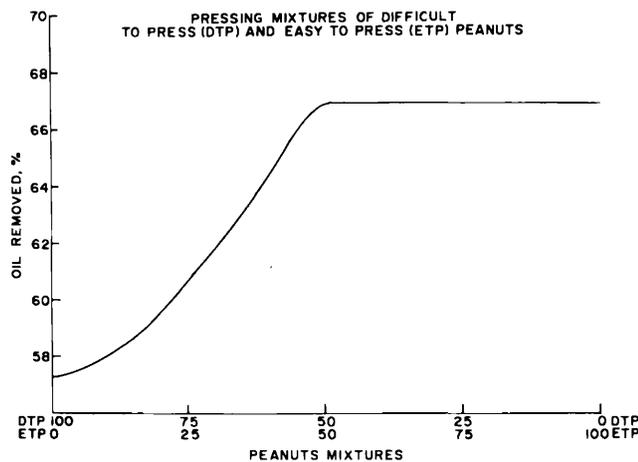
Fig. 1. Effects of Easy-to-Press peanuts on removing oil from Difficult-to-Press peanuts.
