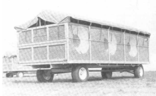
Fig. 1. A wind-powered, natural air drying module.
