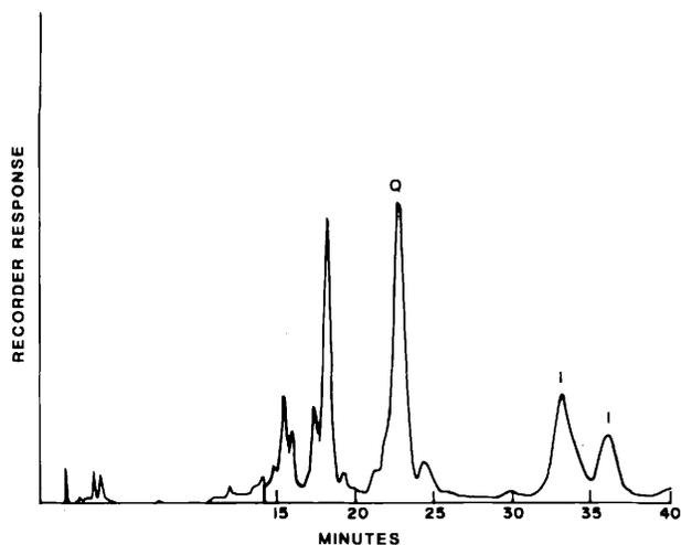
Fig. 2. Chromatogram of Spanwhite skin extract. (Flow rate 2 ml/min, 10 min linear gradient [90-65% of 1% HOAC and 10-35% of methanol] on a 30 cm X 3.9 mm  $\mu$  Bondapak C<sub>18</sub> column). Q = quercetin derivative; I = isorhamnetin derivative.
