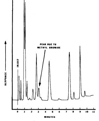
Fig. 1. Chromatogram of the headspace gases after heating peanuts which had been treated with methyl bromide. Arrow shows peak due to methyl bromide treatment which appears in the analysis.
