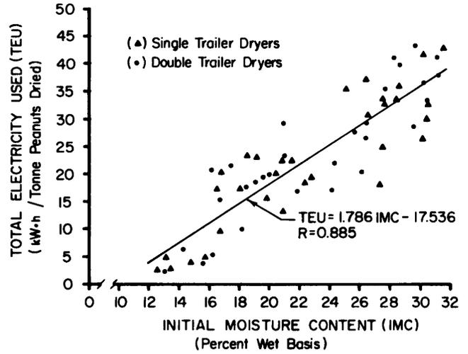
Fig. 2. The effect of initial m.c. on total electricity used for drying peanuts with ST and DT dryers.
