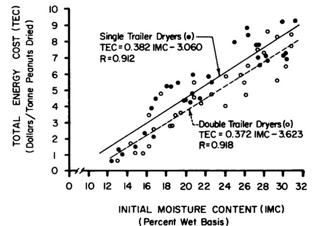
Fig. 4. Comparison of the effects of initial m.c. on total energy costs for drying with ST and DT dryers.
