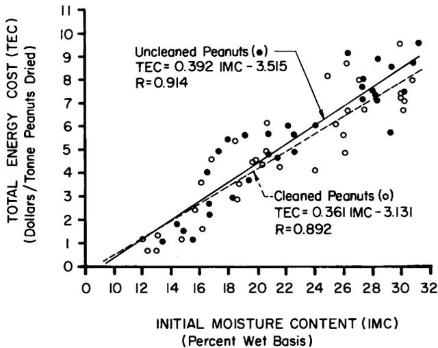
Fig. 8. Comparison to total energy costs for drying Uc and C peanuts.
