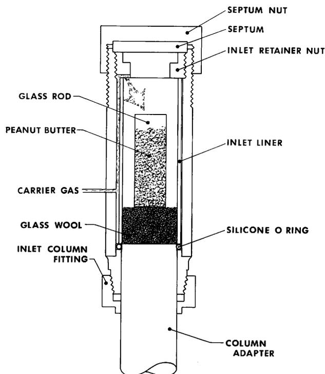
Fig. 1. Cross section of inlet of gas chromatograph with inlet liner containing glass wool and glass rod.
