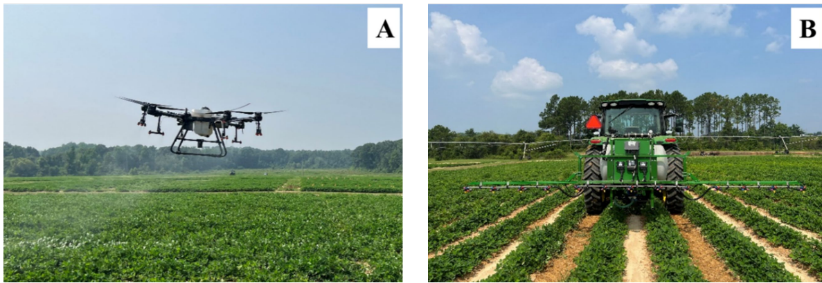
Figure 1. (A) DJI T30 spray drone and (B) LMC boom sprayer used for spray applications in peanut studies conducted in 2023 and 2024.
