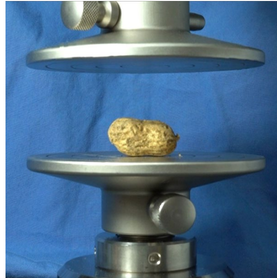
Figure 1. Peanut pod placed in position on lower compression plate for hull rupture testing.
