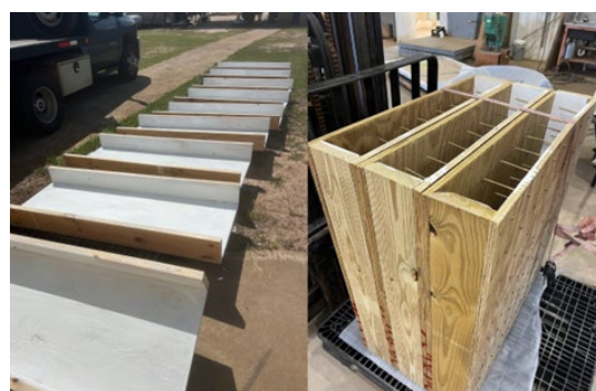
Figure 2. Photographs of root box assembly. Left side displays half assembled boxes with the main wall covered in white paint. Right side displays completed boxes with closed face and nails inserted through the painted white side.
