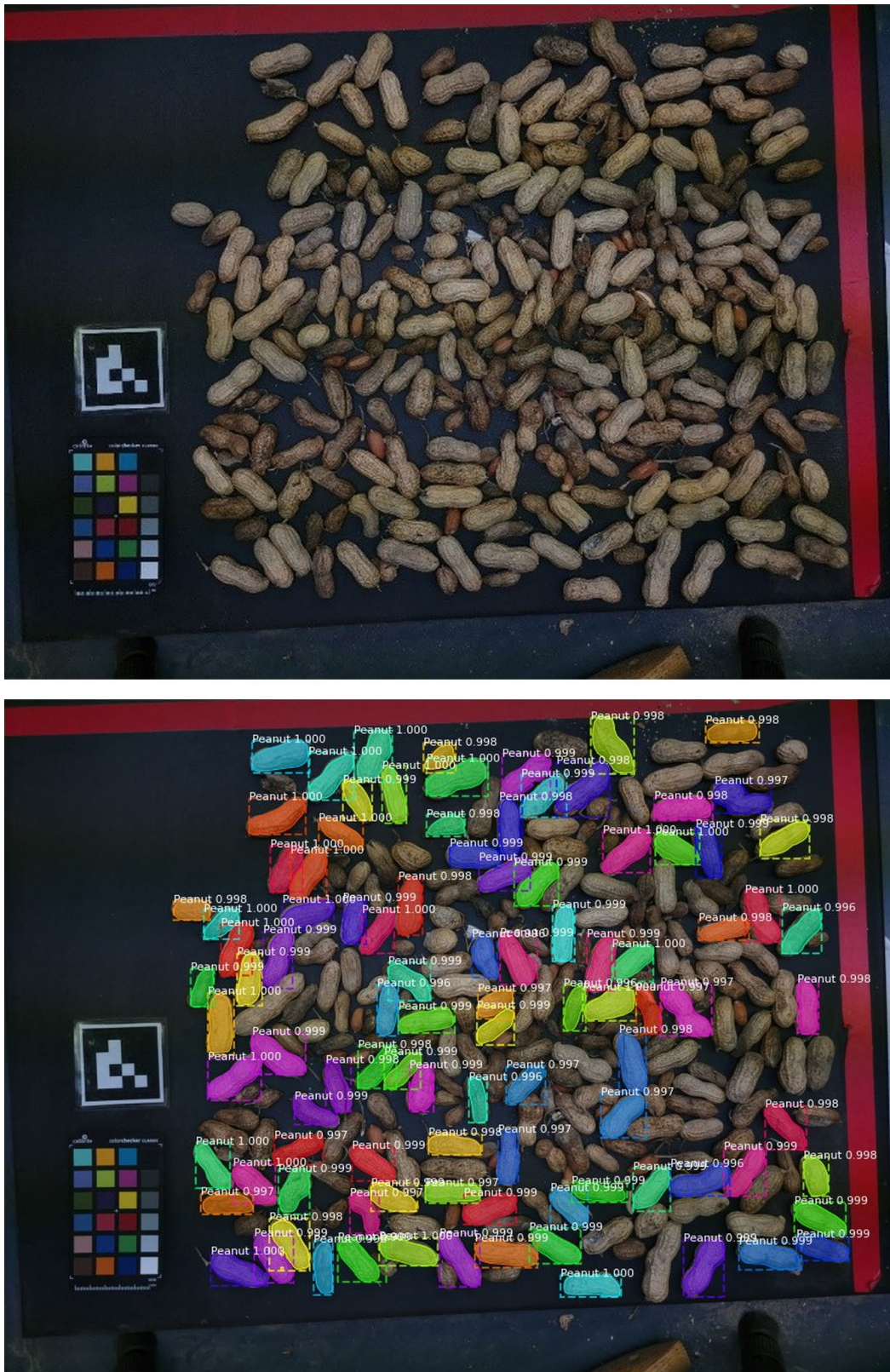
Figure 4. Example of Mask R-CNN input (top) and output (bottom) image on a field sample of the 2022 NCSU advanced yield trial. Each of the 100 detected pods is shown in a distinct color in the bottom image which represents their respective segmentation mask. All 100 detections are pods and no loose shelled kernel (LSK), stick, rock or other detritus were masked in a distinct color.
