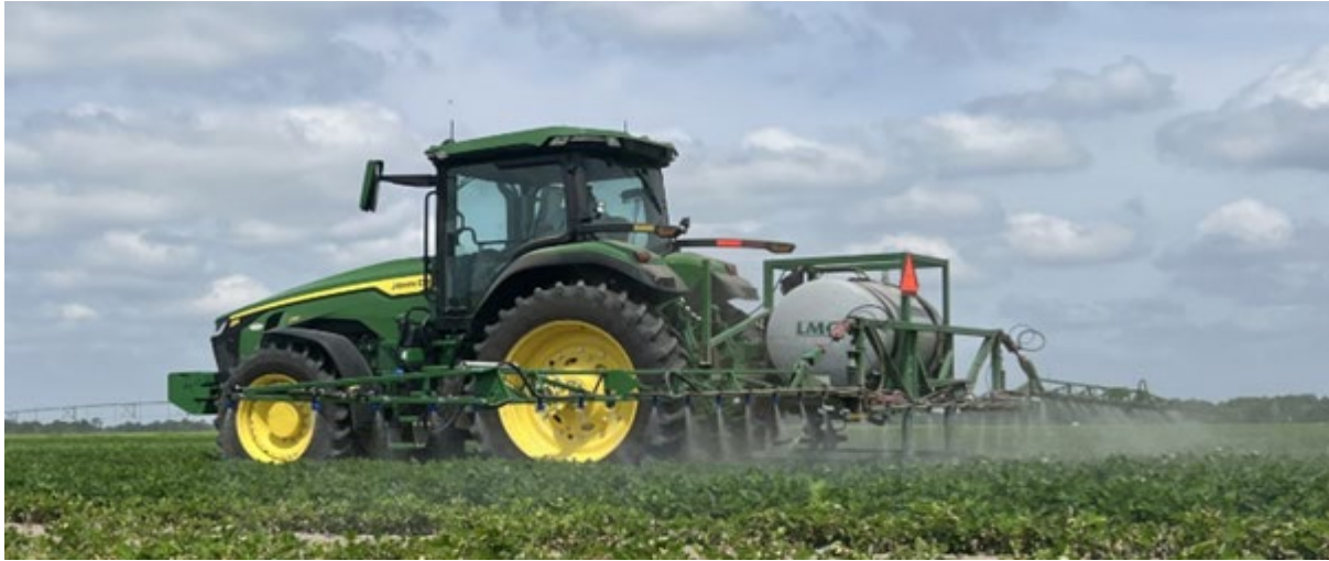
Figure 1. The commercial LMC boom sprayer used for herbicide applications in the peanut spray studies conducted in 2021 and 2022.
