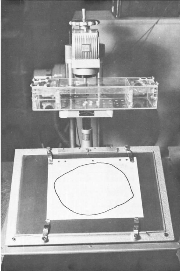
Fig. 1. Wilder Microprojector Equipped with 20X Lens and Environmental Chamber for Drying Peanuts.
