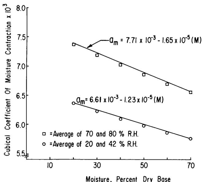
Fig. 2. Cubical Coefficients of Moisture Contraction and Regression Lines as a Function of Moisture Content and Drying Air Relative Humidity.
