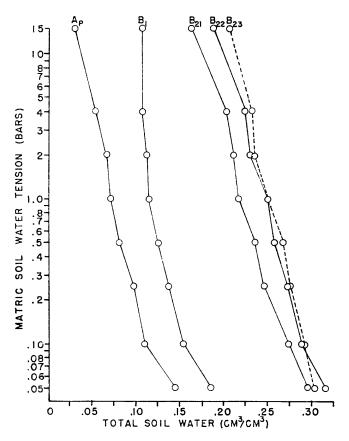
Fig. 2. Water retention curves for Tifton loamy sand.
