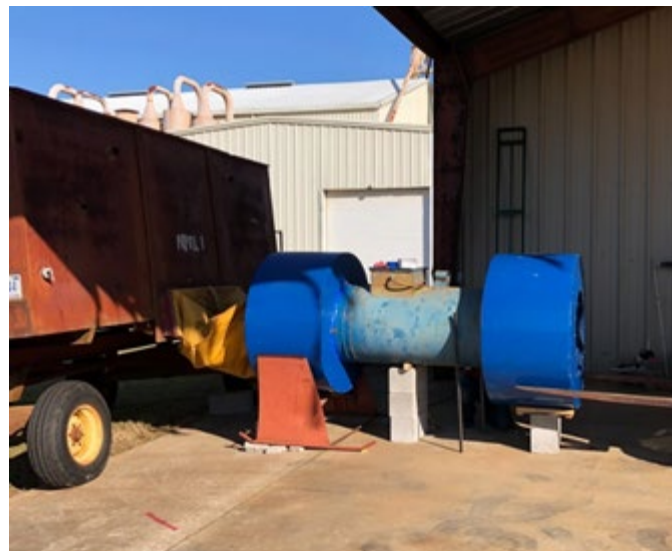
Figure 2. Peanut dryer with 1.17m cylindrical dark blue fiberglass lined mufflers attached to the air intake and exhaust of lighter blue peanut dryer. Muffler on dryer air exhaust is attached by a yellow vinyl air duct to a trailer loaded with in-shell peanuts.
