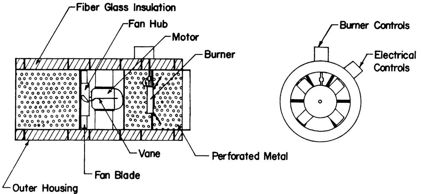
Fig. 5. Redesigned fan-burner unit.
