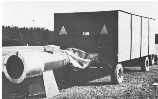
Fig. 2. Muffler mounted on inlet of fan-burner unit in position for SPL tests.
