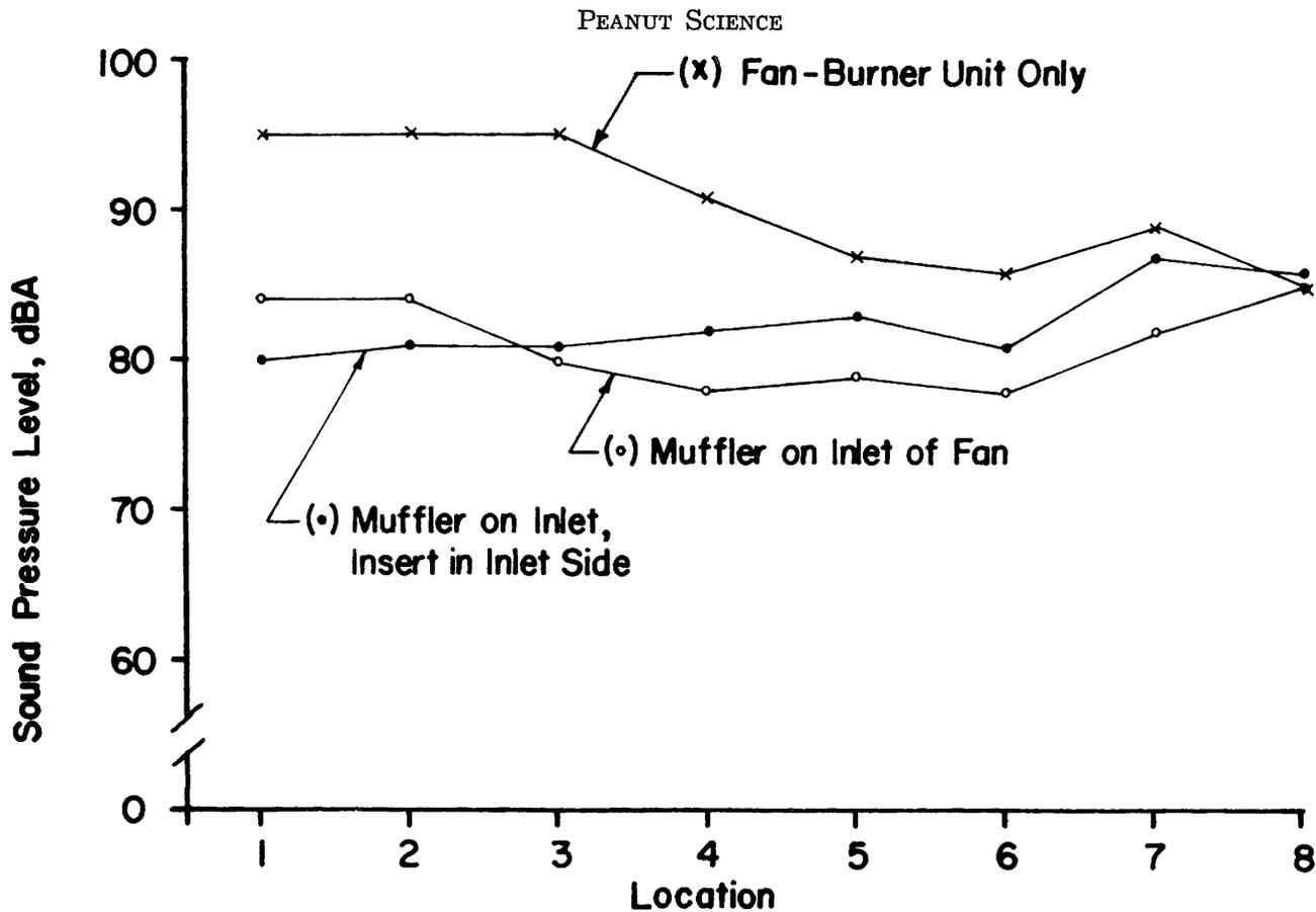
Fig. 3. Sound-pressure levels after inlet of fan-burner unit received acoustic treatment.
