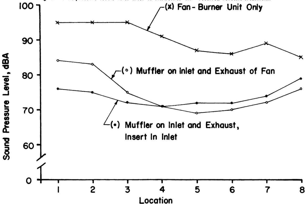
Fig. 4. Sound-pressure levels after inlet and exhaust of fan-burner unit received acoustic treatment.
