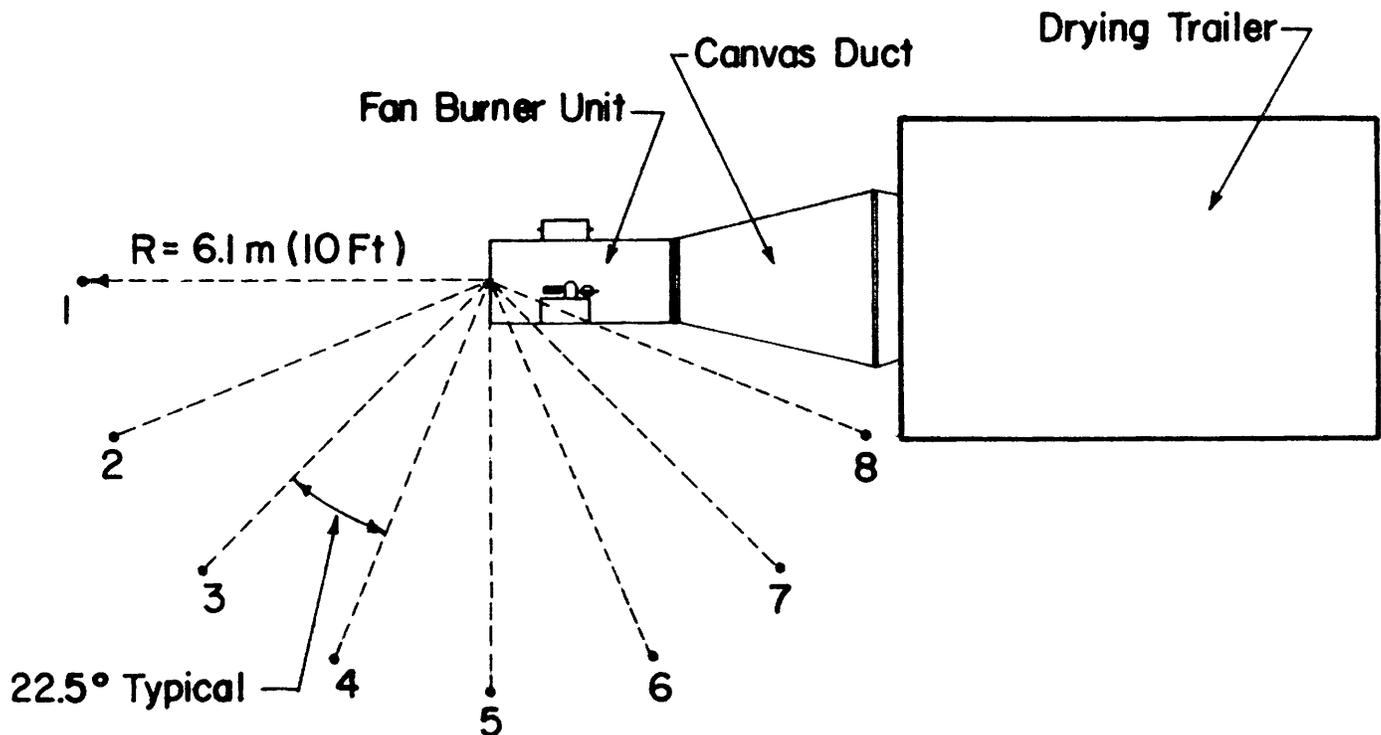
Fig. 1. Location of measurement positions for SPL tests.
