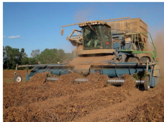
Fig. 4. An 8-row self-propelled peanut combine manufactured as a joint venture between Amadas Industries and John Deere (photo provided by Amadas Industries, Suffolk, VA).
