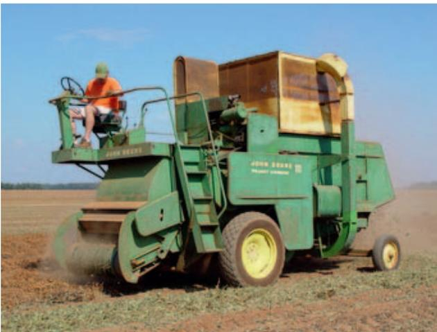
Fig. 2. John Deere two-row self-propelled peanut combine circa 1964 (picture used by permission)
