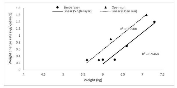
Fig. 5. Drying rate of single-layer solar drying and simultaneous open sun drying.
