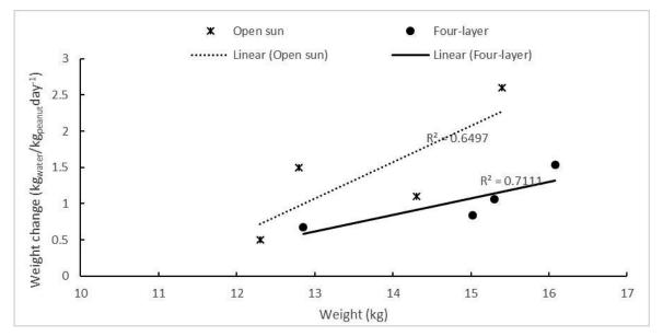
Fig. 6. Drying rate of four-layer solar drying and simultaneous open sun drying.
