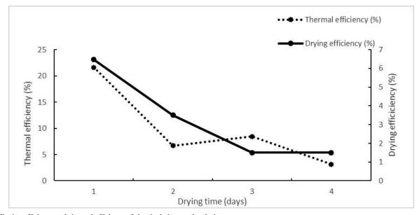
Fig. 8. Drying efficiency and thermal efficiency of the single-layer solar drying.
