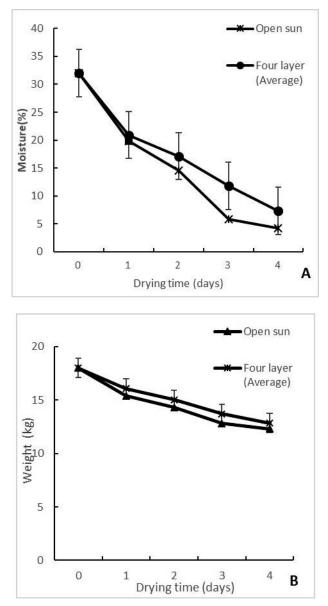
Fig. 4. Moisture (A) and weight (B) of peanuts in the four-layer solar drying and simultaneous open sun drying.
