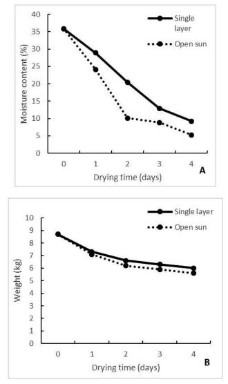
Fig. 3. Moisture (A) and weight (B) of peanuts in the single-layer solar drying and simultaneous open sun drying.
