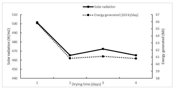
Fig. 7. Average solar radiation absorbed by the solar collector and daily energy generated by the solar dryer during the single-layer solar drying.
