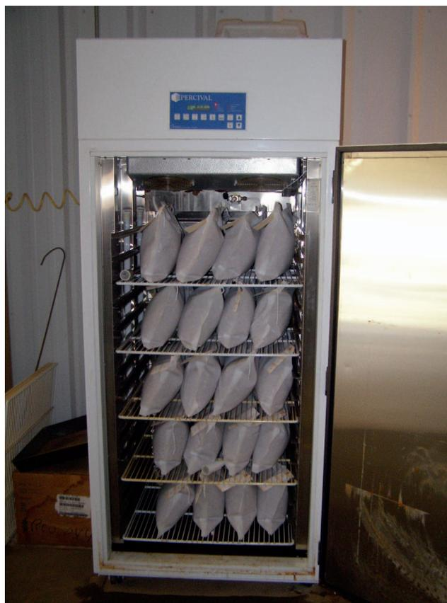
Fig. 2. Placement of samples in controlled environment chamber for studies to determine effect of storage conditions of chemical, sensory, and germination characteristics of shelled peanuts.
