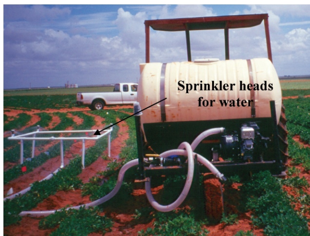
Fig. 1. Device used to apply water over the top of fungicide treated plots, to simulate chemigation. The device was constructed by T. Wheeler and D. Porter.
