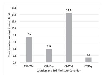
Fig. 2. Time needed between wetting events under different soil moisture conditions on conservation production system and conventional tillage fields growing peanuts. The numbers shown over the bars indicates the d needed between wetting events to maintain soil moisture in the 50 to 80 kPa range. CSP is the conservation production systems field in Bulloch County and CT is the conventional tillage field in Worth County. Wet is the condition of the soil moisture potential is below 50 kPa.
