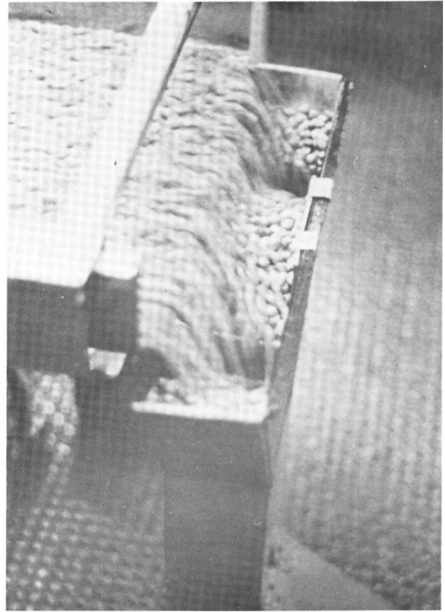
Fig. 14. Photograph of chute with baffles installed to entrap peanuts.
