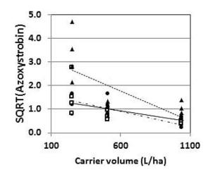
Fig. 3. The relationship between foliar transformed (square root) azoxystrobin concentration (A) in ppm and carrier volume (V), applied at three different times during the season (24 July; 7 Aug; 16 Aug). The equations fitted for each application time were: 24 July  $-\!\!\!/ \sqrt{A} = 1.48 - 0.00091(V), R^2 = 0.49$ 7 Aug  $-\!\!\!/ \sqrt{A} = 1.70 - 0.0013(V), R^2 = 0.43$ 16 Aug  $\cdots \sqrt{A} = 3.31 - 0.0025(V), R^2 = 0.46$ .
