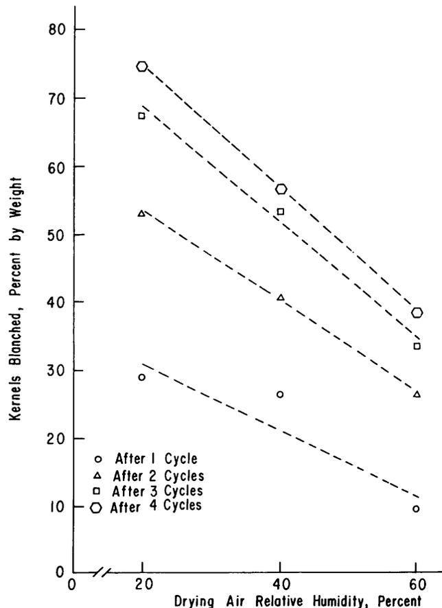
Fig. 2. Effect of Drying Air Humidity on Peanut Kernels Blanched (Each Point is the Mean of Three Runs).
