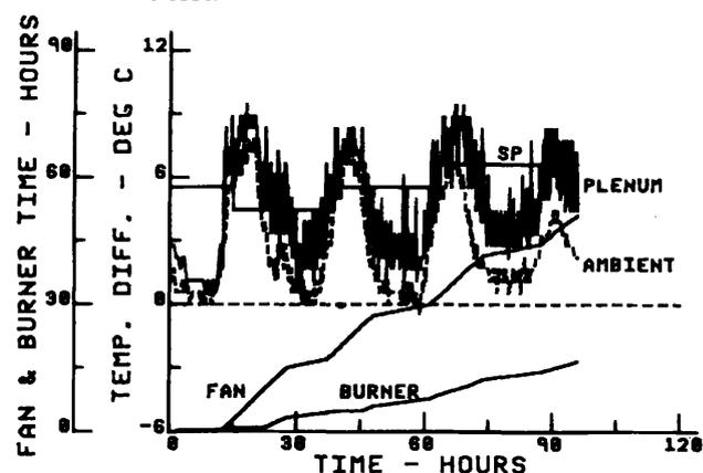
Fig. 6. Plenum and ambient wet bulb depressions, set point depression and fan and burner operating time vs time on the dryer for ECT2, 1980.
