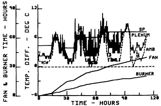
Fig. 4. Plenum and ambient wet bulb depressions, set point depression and fan and burner operating time vs time on the dryer for ECT1, 1980.
