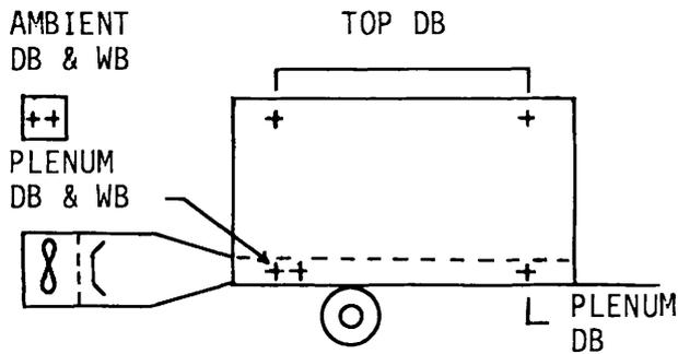
Fig. 2. Dry bulb (DB) and wet bulb (WB) thermocouple locations for peanut dryer control and performance data.
