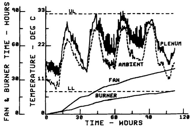
Fig. 3. Plenum and ambient temperature, upper and lower limits and fan and burner operating time vs time on the dryer for ECT1, 1980.
