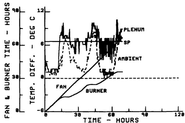
Fig. 5. Plenum and ambient wet bulb depressions, set point depression and fan and burner operating time vs time on the dryer for CONV1, 1980.
