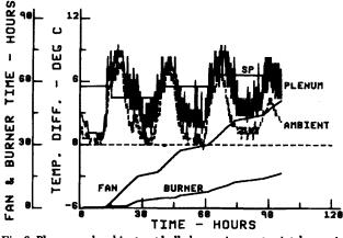
Fig. 6. Plenum and ambient wet bulb depressions, set point depression and fan and burner operating time vs time on the dryer for ECT2, 1980
