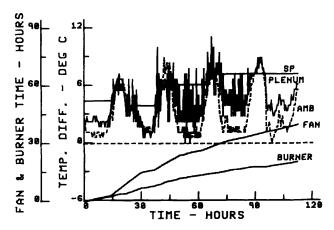
Fig. 4. Plenum and ambient wet bulb depressions, set point depression and fan and burner operating time vs time on the dryer for ECT1, 1980.
