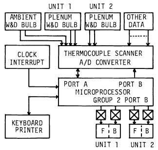
Fig. 1. Block diagram of microprocessor based peanut dryer control system.
