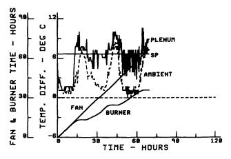
Fig. 5. Plenum and ambient wet bulb depressions, set point depression and fan and burner operating time vs time on the dryer for CONV1, 1980.
