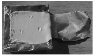
Fig. 1. Shape of the final sample obtained after transformation of the raw products according the process described in the text (Shearing duration = 2 min) (zoom x2).
