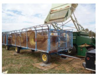
Fig. 4. The peanut wagons and truck scales that were utilized to weigh each calibration and yield load in the field during harvest.
