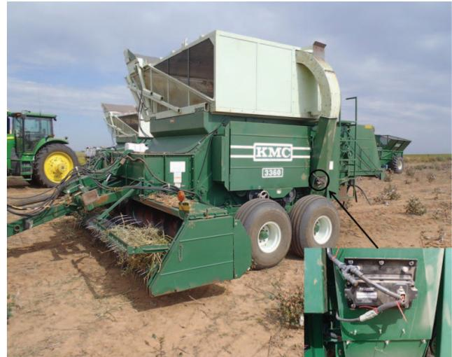
Fig. 1. The mounting location of the AgLeader Yield Monitor on a KMC 6-Row Peanut Combine.
